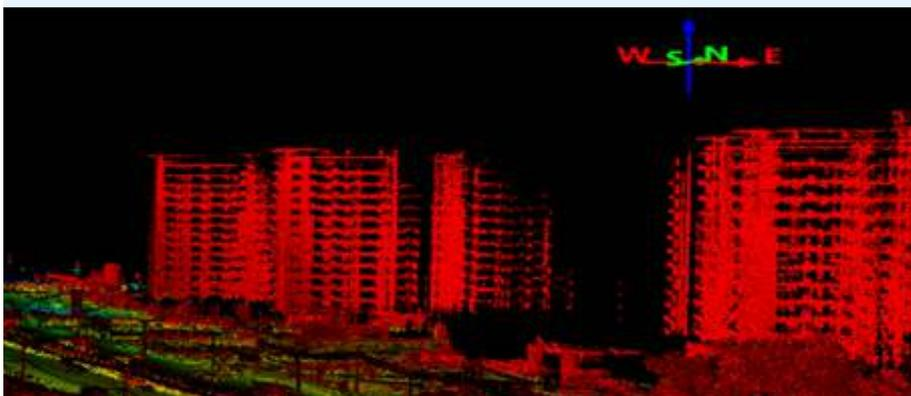
The working principle is similar to Aerial application, the only difference being the LiDAR Payload is mounted on a ground vehicle. The pulsed laser beam is reflected from objects such as building fronts, lamp posts, vegetation, cars and even people. The return pulses are recorded and the distance between the sensor and the object is calculated.
