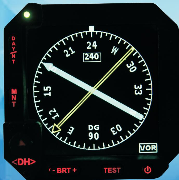
The RADIO MAGNETIC INDICATOR (RMI) is used on Cheetah/ Chetak helicopters to provide the Heading and VOR bearing, by interfacing with Gyro Compass (or AHRS) and VOR. The electrical interfaces are ARINC-429 and Discrete I/Os. The unit avoids interfaces like Synchro or Resolver and thereby provides easy wiring, scalability and ease of maintenance. It is equipped with a 3-ATI AMLCD display with LED back-light.
