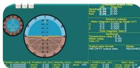
The DILABS INS utilizes advanced single and dual antenna GNSS receiver, barometer, 3-axes each of calibrated in full operational temperature range precision Fluxgate magnetometers, Accelerometers and Gyroscopes to provide accurate Position, Velocity, Heading, Pitch and Roll of the device under measure. INS contains DILABS new on-board sensors fusion filter, state of the art navigation and guidance algorithms and calibration software.
